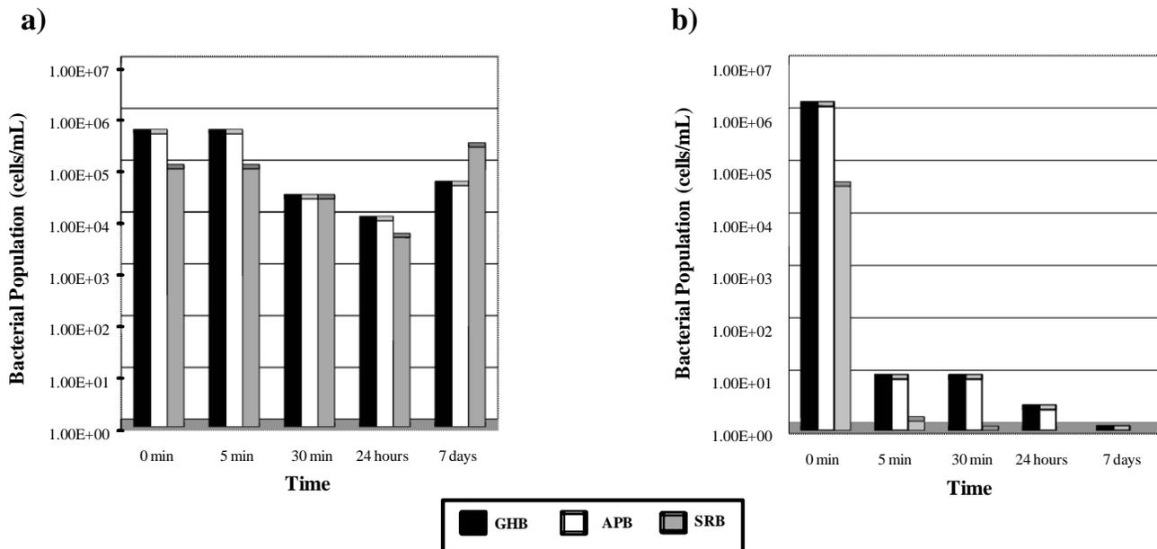
**Figure 1** Laboratory bacterial test results, including a) 263 ppm glutaraldehyde in the Piceance Basin water sample and b) the 5 ppm oxidative biocide in the Piceance Basin water sample, over a seven day period. The Piceance Basin water sample was tested and had a pH value of 8.06 and a total dissolved solids concentration of 143,000 ppm.
