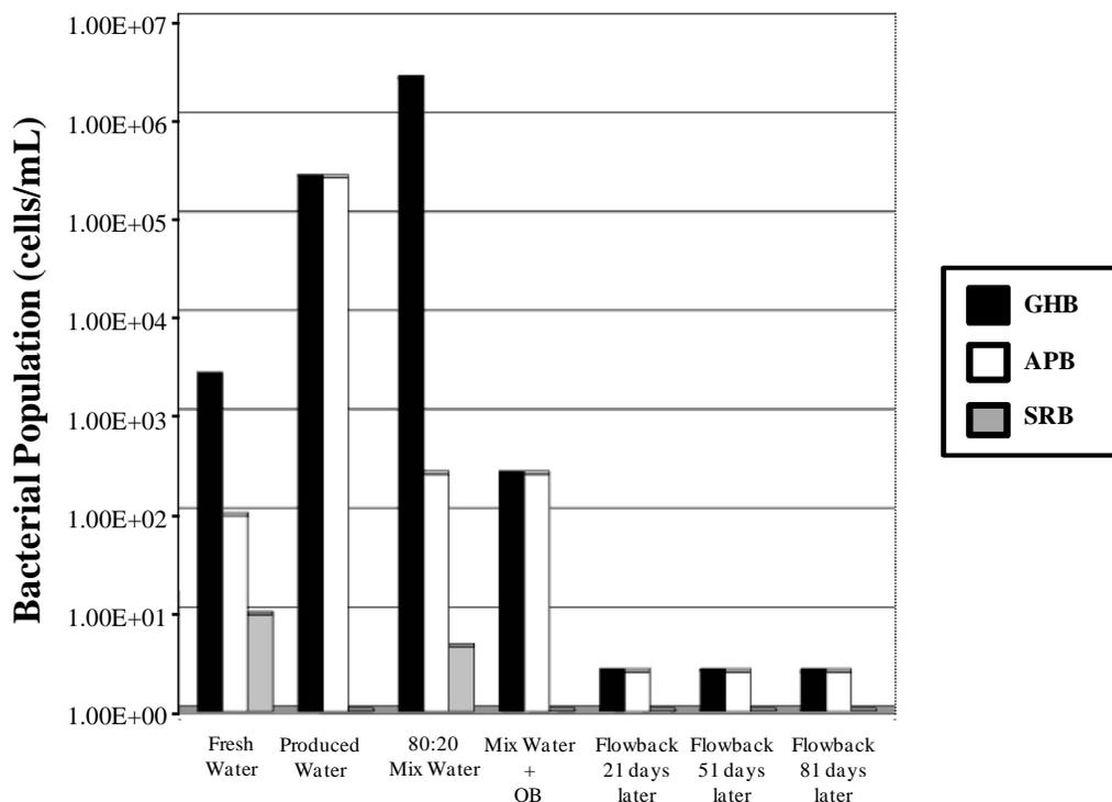
**Figure 5** Bacterial test results, including fresh and produced water, an 80/20 mixture of PW and FW, and flowback samples from the well.
