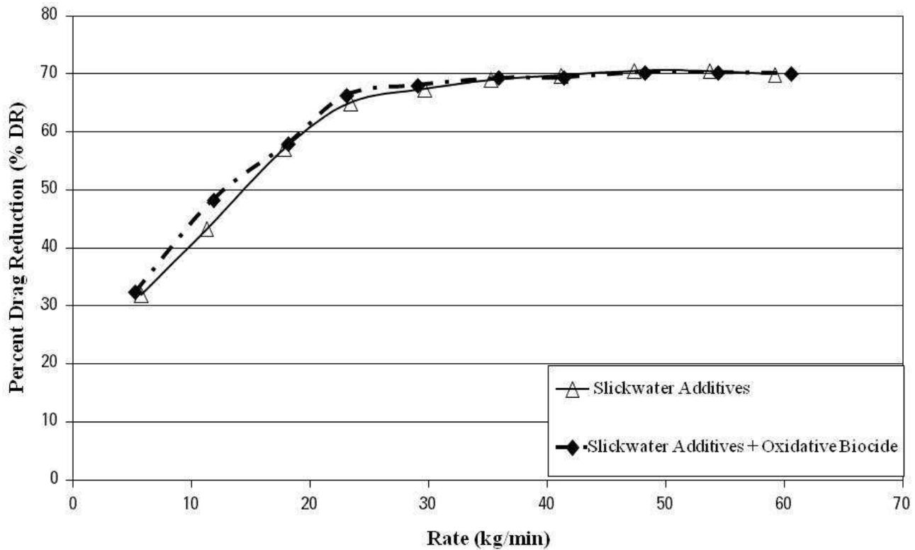
**Figure 2** The maximum percent drag reduction (%DR) value for the Piceance Basin (PB) water sample containing slickwater additives (2000 ppm clay stabilizer, 275 ppm friction reducer, 109 ppm scale inhibitor, and 1818 ppm microemulsion solvent and PB water sample) and 5 ppm oxidative biocide. The Piceance Basin water sample had a pH value of 8.06 and 143,000 ppm TDS.
