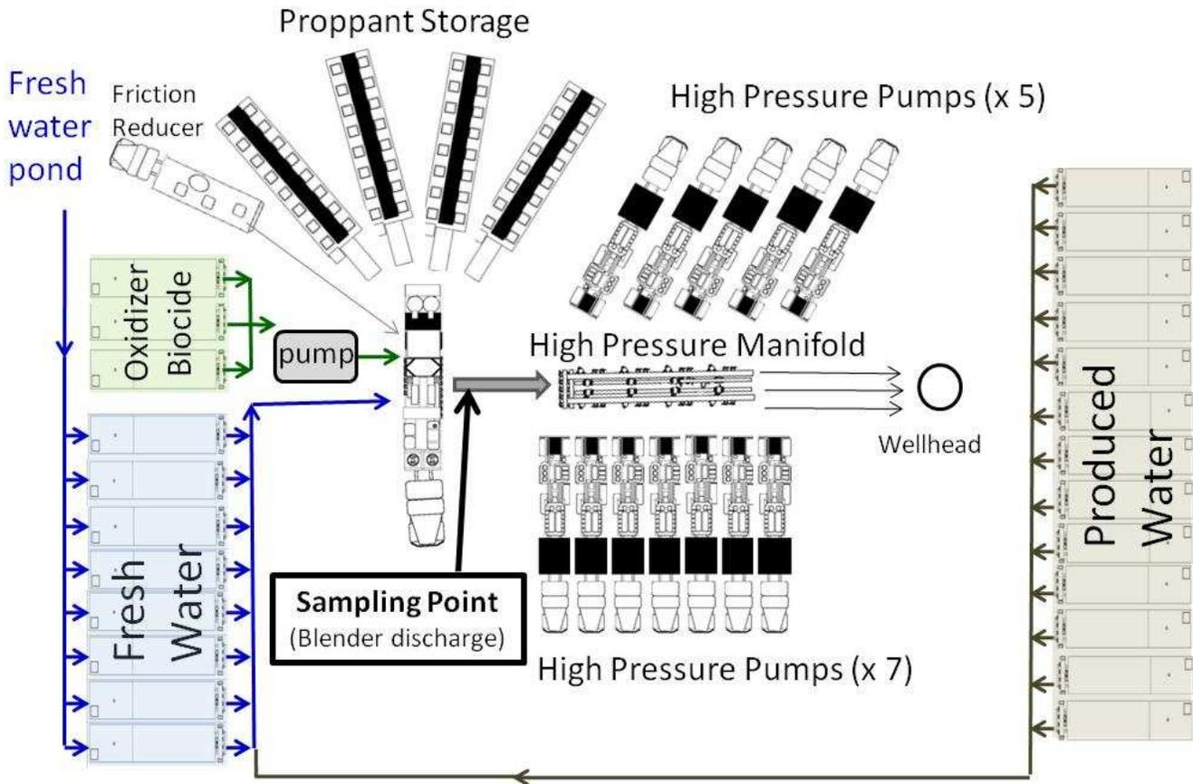
**Figure 4** Schematic of the wellsite in this case study. Water was sampled from the fresh and produced water tanks, and from the blender.
