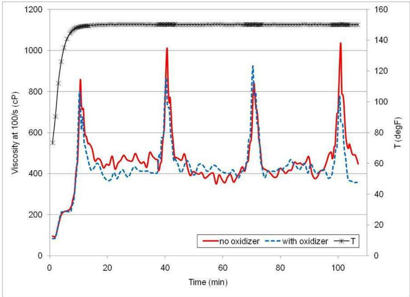
**Figure 3** Rheology profile of a crosslinked 20 lb guar gel at pH 11.25 with 5 ppm oxidative biocide at 150 °F.
